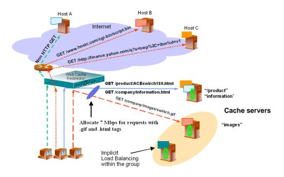
Figure 17-5 URL-Based Bandwidth Management with Web Cache Redirection
